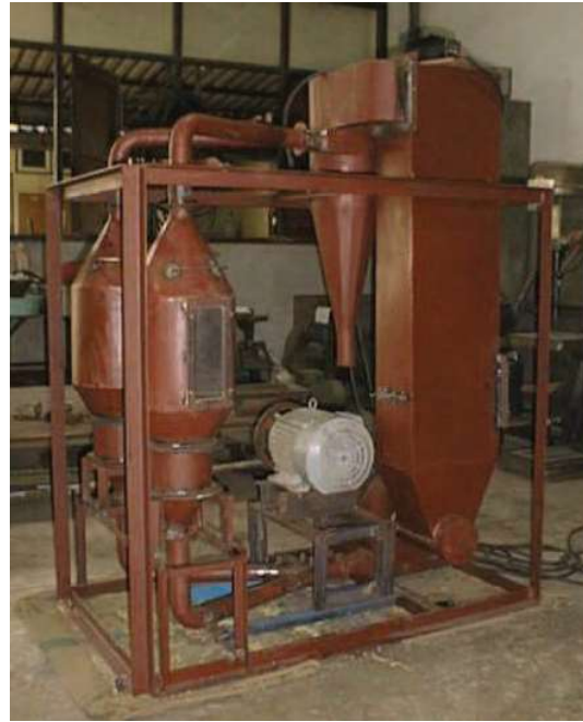
Figure 4 Prototype of rapid dryer for wet grain
