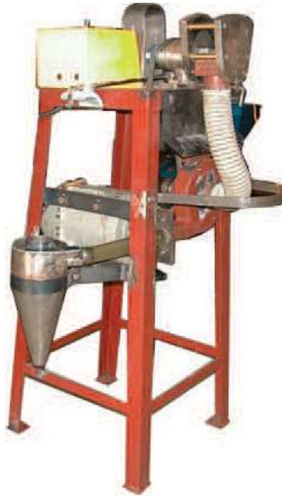
Figure 3 Prototype of friction-type paddy milling quality determination instrument.
